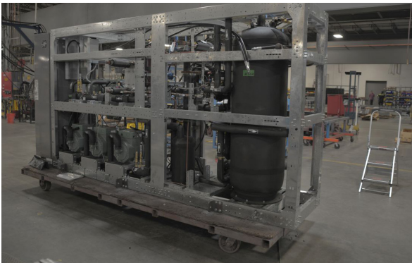
Figure 3-5. Rack system mounted on the ground
